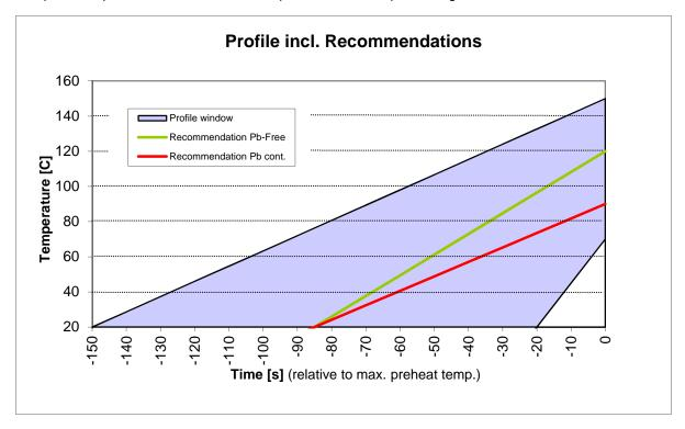
**DO NOT:** Use too high pre-heat temperatures as this will degrade the flux performance.
